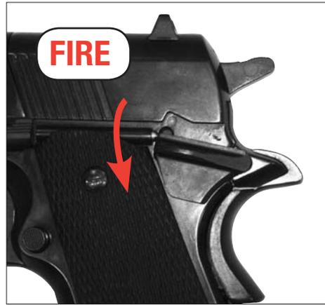
To release the safety, push the lever down.
