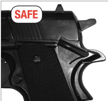
The pistol cannot fire if the grip safety is not pressed.
